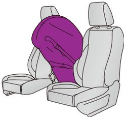
Driver's seat has a far side airbag in addition to the side airbag. Location of far side airbag is shown in the mark 9. on page 1.
